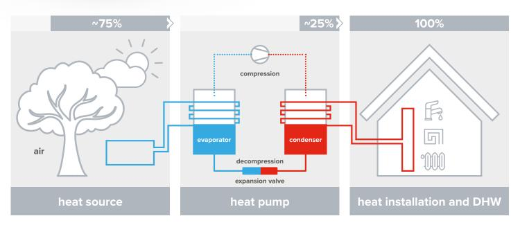
The operation of a heat pump can be described as reversed operation of a fridge. Heat is always transferred from the warmer to the colder item. This principle is used, and that is why pumps operate. Just like a fridge transfers the heat from the inside and moves it outwards, heat pump removes the heat from the external area and transfers the energy inside the home in the
